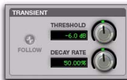
Time Shift plug-in, Transient section with Rhythmic selected as the Audio Type
